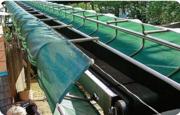
Machinery Safety Barriers for Water Park Conveyer Belt
