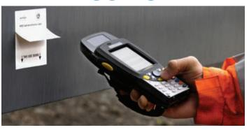
ARG has the ability to install an RFID chip on every sling or piece of rigging hardware we fabricate or test. This will allow you to easily identify each asset and access its associated documents and certifications through our online portal. You have 24/7 access and can print certs, see exactly when the asset was made and how long it has been in service, and the last time it was tested and or inspected.
