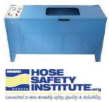
NAHAD suggest that each new assembly gets pressure tested to one and half times the maximum working pressure before they are put into use. ARG can test and certify assemblies up to 30,000 psi.
